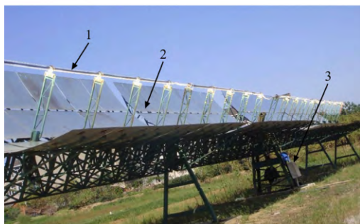
1. 真空集热管 2. 抛物槽式聚光镜 3. PLC控制柜 1. Evacuated collector tube 2. Parabolic trough concentrating mirror 3. PLC control cabinet
